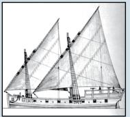
and stern, and propelled by oars or by sail in light winds. They were built to carry a heavy cannon in the bow, flanked by smaller cannon and swivel guns, and measured about 70 feet long. Twenty double-manned oars on each side required at least 80 seamen who stood upright to row. Troops from the Continental Line were drafted to serve as marines.
